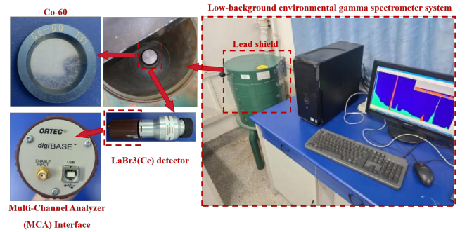
Fig. 6. (Color online) Low-background environmental gamma spectrometer system and Co-60
